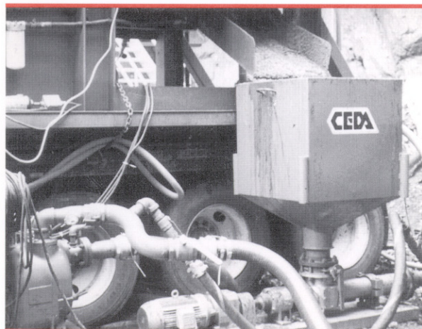
Sludge handling equipment for full-scale trial
