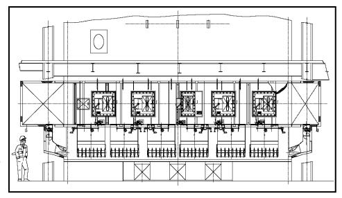
The units were still operated with the original combustion air delivery systems consisting of primary air and tangential upper secondary air; cascade direct contact evaporators are also in use.
