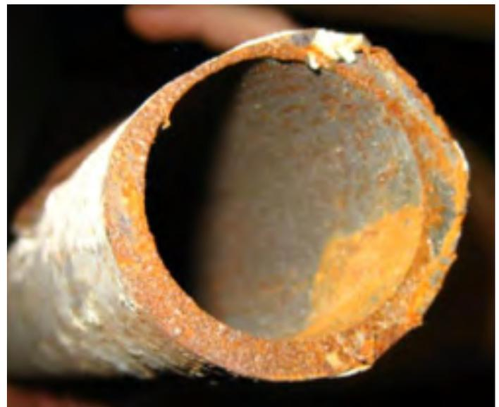
*Photo of a severely eroded boiler tube.*
