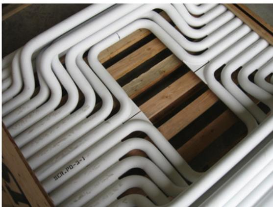
Jansen-Designed Wall Tube Panel for Fuel Distributor Opening
