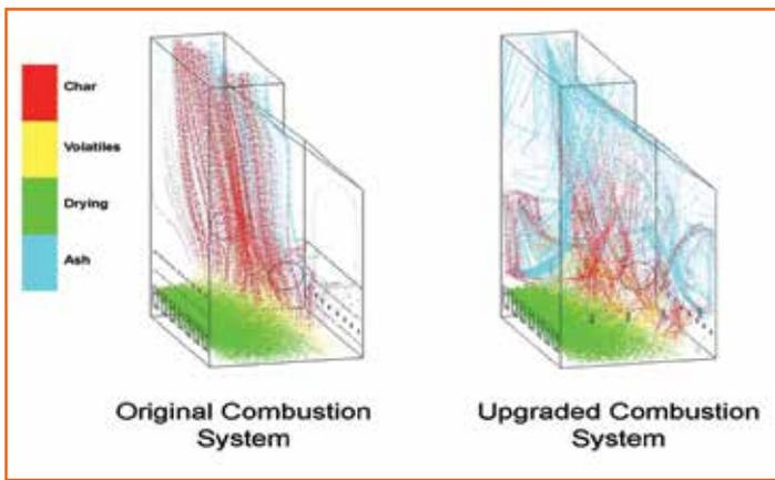
Figure 4: Improvement in the burnout in the in-flight fuel particles by improved air and fuel delivery
