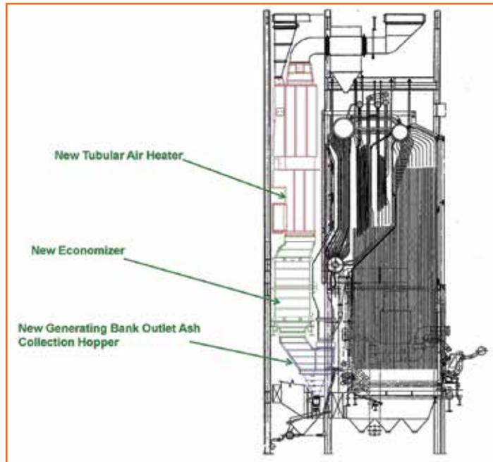
Figure 5: The modified GB outlet ash collection hopper that was installed on the boilers to reduce the flue gas velocities through the 180° turn and improve the drop out of fly ash into the hopper
