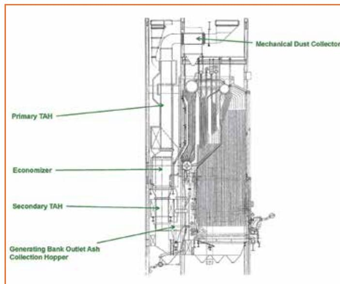
Figure 1: A sectional side view of the boilers following the 1985 conversion
