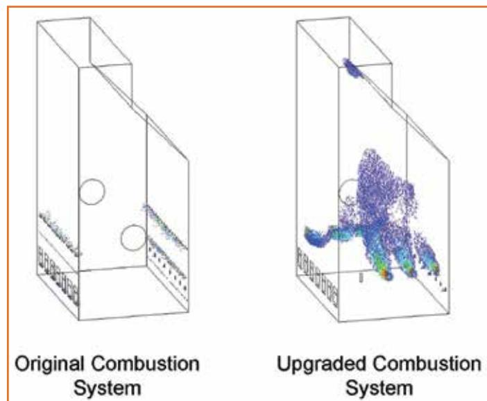
Figure 3: Modelling plots of the jet penetration profiles of the original and upgraded combustion systems, where regions of the furnace with velocities higher than 18m/s are shown
