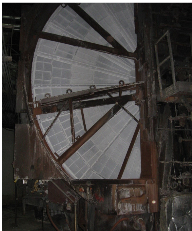
Laminar Air Heater Wheel with Salt Cake Deposition
